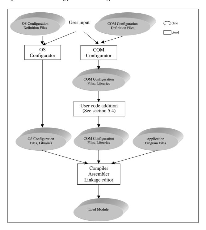
Figure 4.1 Building Process of a COM Application.
