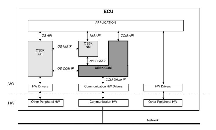
Figure 1.2 Internal SW Structure of an ECU
