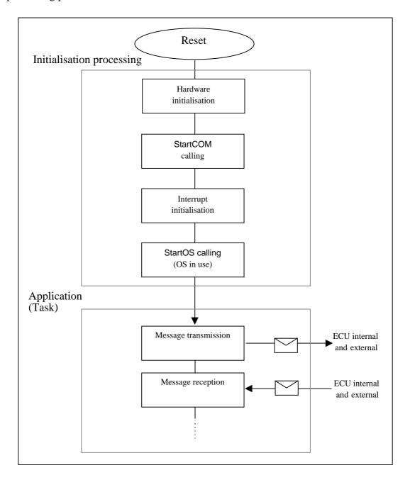
Figure 3.5 COM Processing Procedure
